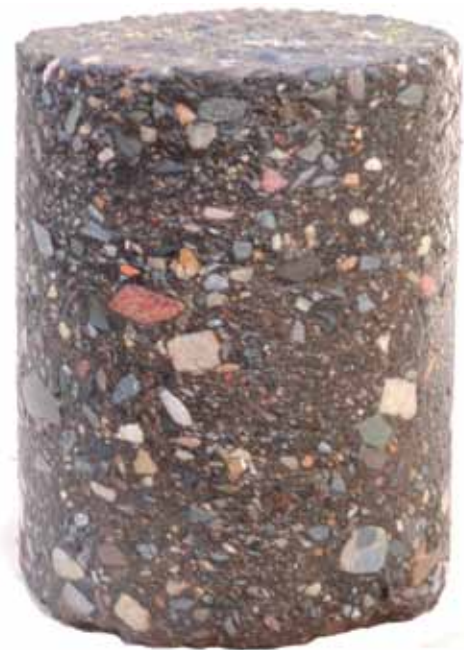
BITUMIX™ core sample cut from a completed roadway.
