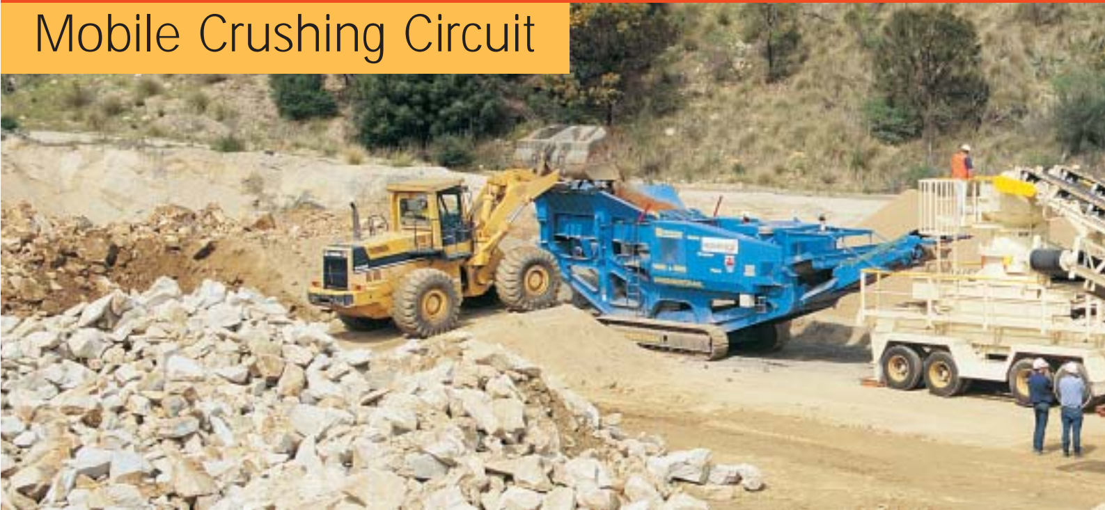
42-30 Pegsun Jaw Crusher feeding
